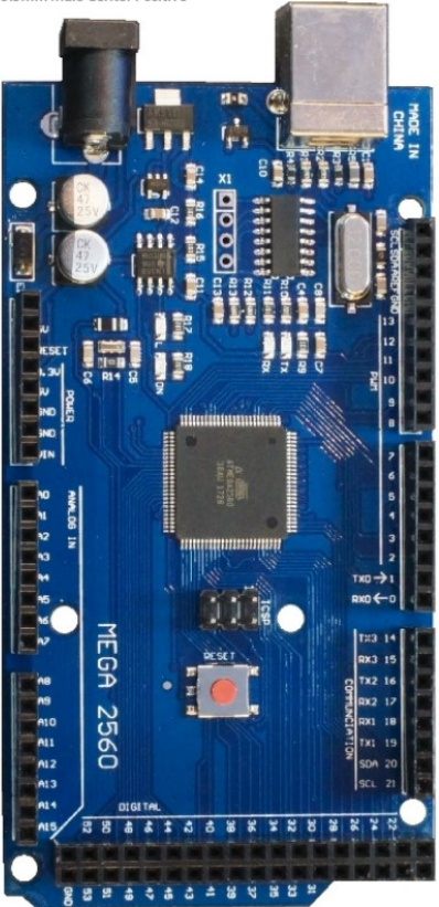
DC Power Jack 7-12VDC Input 2.1mm x 5.5mm Male Center Positive USB-B Port To Computer
