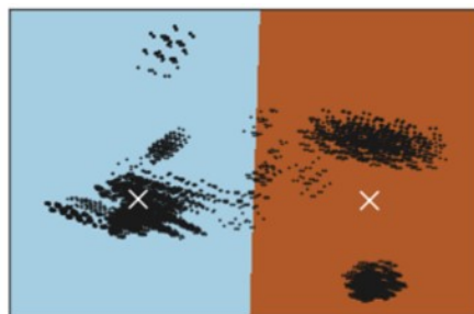
Figure 2.2: Voronoi diagram with clusters (centroids are marked with white cross)
