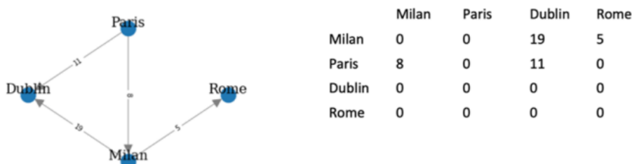
Figure 3.5: Example of an edge-weighted, labeled DiGraph and its adjacency matrix [10]
