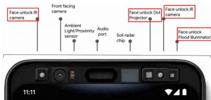
Figure 3.2: Modules involved in face recognition of the Google Pixel 4 [62]
