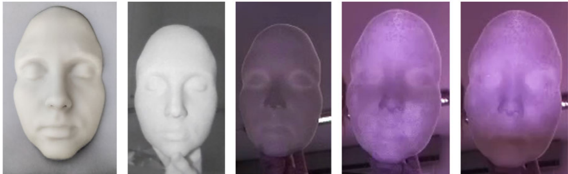
Figure 3.42: Resin mask (left), the mask's appearance in HedgeCam2 (second from left), the Google Pixel 4's point cloud (middle) and the Apple iPhone 12's point clouds (second from right and right)
