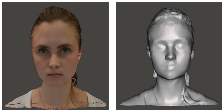
Figure 3.46: Model with texture generated with SfM (left) and model without texture captured with SfM (right)
