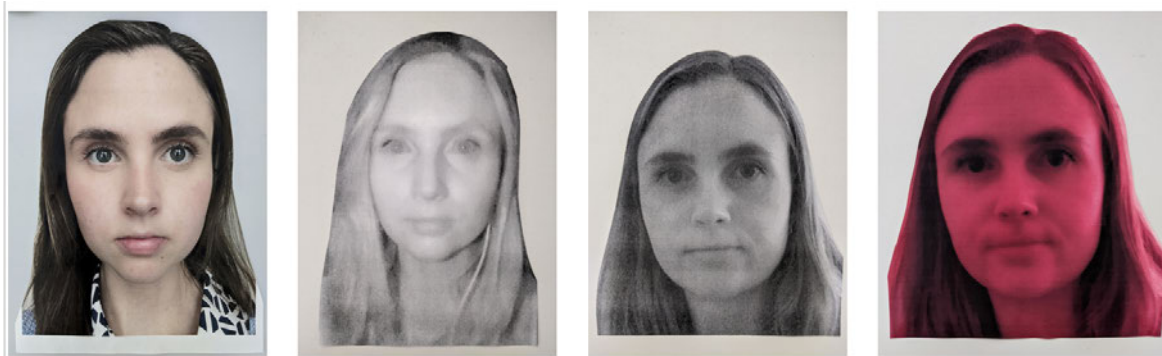
Figure 3.29: Printed artefacts captured with the RGB camera (left), captured with HedgeCam2 (second from left) and captured with the IR camera of the Raspberry Pi printed without (second from right) and with colour (right)
