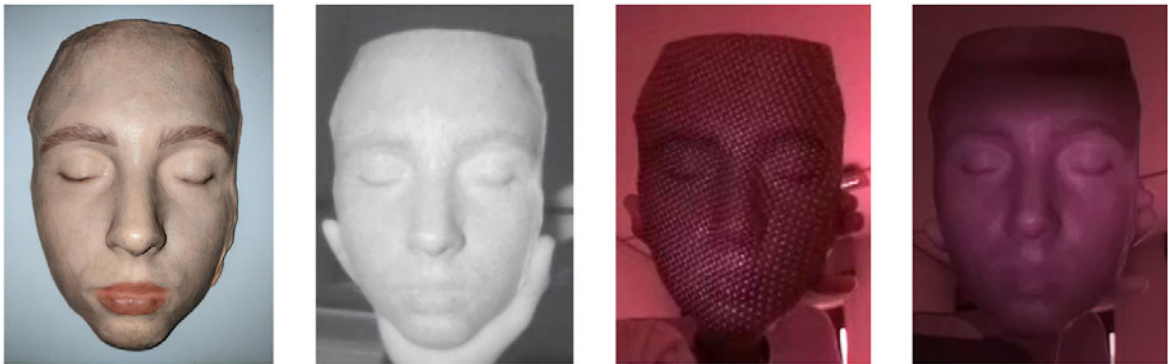
Figure 3.37: Mask with applied makeup (left), its appearance in HedgeCam2 (second from left), the Google Pixel 4's point cloud (second from right) and the Apple iPhone 12's point cloud (right)
