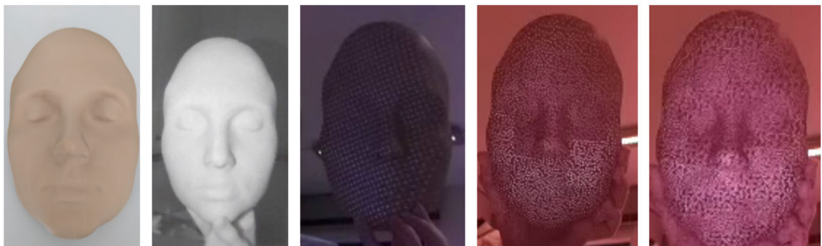
Figure 3.40: Printed mask (left), the mask's appearance in HedgeCam2 (second from left), the Google Pixel 4's point cloud (middle) and the Apple iPhone 12's point clouds (second from right and right)
