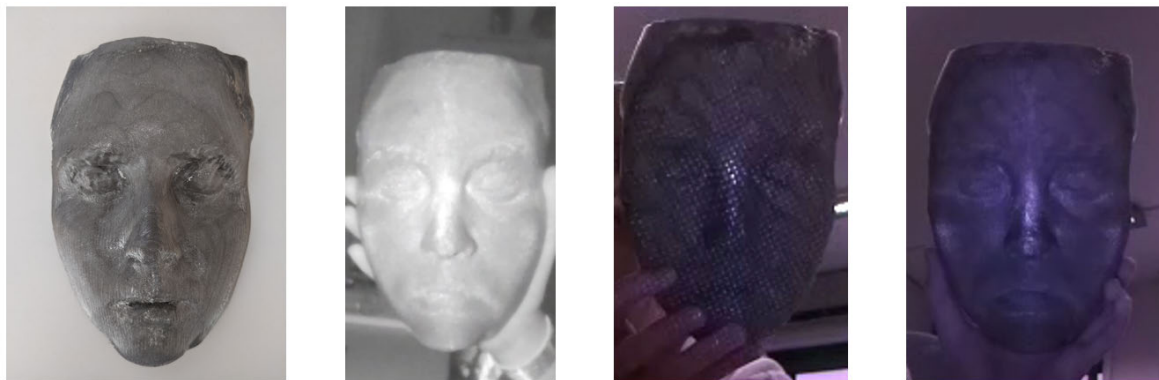
Figure 3.36: Printed mask with grey PLA (left), mask's appearance in HedgeCam2 (second from left), mask's point cloud from the Google Pixel 4 (second from right) and mask's point cloud from the Apple iPhone 12 (right)
