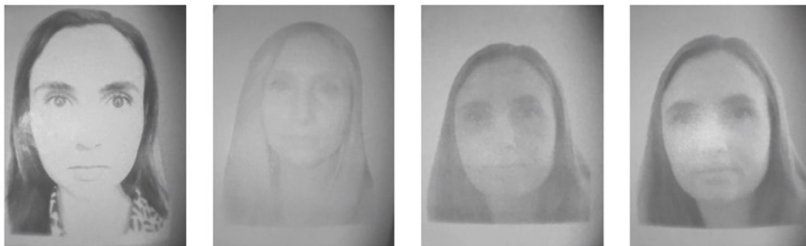
Figure 3.30: Appearance of the two-dimensional artefact captured with the RGB camera (left), captured with HedgeCam2 (second from left) and captured with the IR camera of the Raspberry Pi printed without (second from right) and with colour (right) in NIR with HedgeCam2
