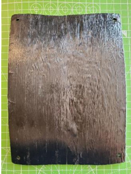
Abbildung 21: 1_Allgemeines Muster_UD-Tape_1 in MCP1223 PA6 CF_#1
