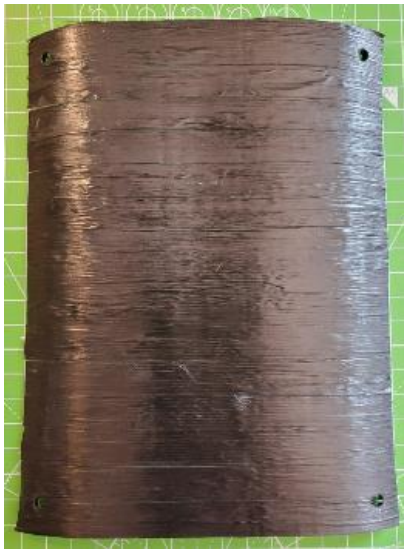
Abbildung 51: 1_Allgemeines Muster_UD-Tape_1 in MCP1223 PA6 CF #1
