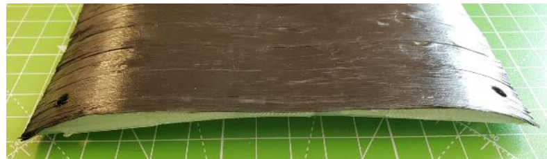
Abbildung 53: 1_Allgemeines Muster_UD-Tape_1 in MCP1223 PA6 CF #2
