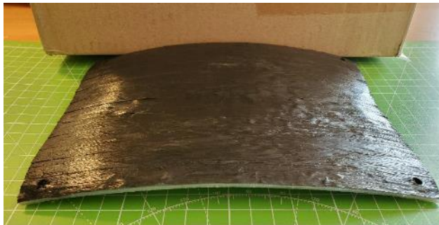
Abbildung 23: 1_Allgemeines Muster_UD-Tape_1 in MCP1223 PA6 CF_#2
